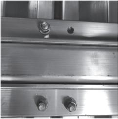
2. Place the HITCH TUBE between the SUPPORT ANGLES and align the holes. Attach it using 3.5" HEX BOLTS, two FLAT WASHERS (one per side), LOCK WASHERS, and HEX NUTS.
