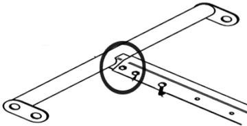
2. Using the WIRE LOCK PIN, connect the SUPPORT TUBE to the LOWER TUBE.
